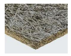
Thermal and acoustic insulation board, specific for external insulation covering, consisting of mineralized fir wood wool bound with grey Portland cement. Wood wool is 3 mm wide. It complies with EN 13168 standard. The boards are certified by ANAB-ICEA and natureplus for eco-compatibility of materials and manufacturing process. CELENIT N/C is PEFC™ certified. Also available with FSC® certification.
