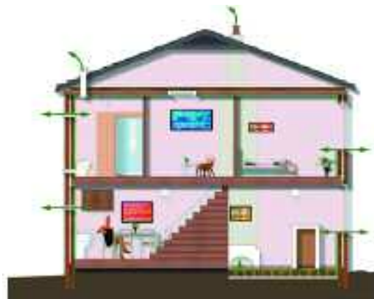
Figure 2 A comfortable well sealed, well ventilated house The key is to build tight and ventilate right.
