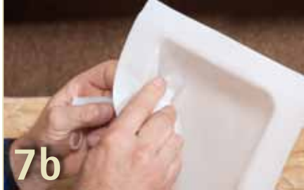
Enlarging: Piercing/pulling through
