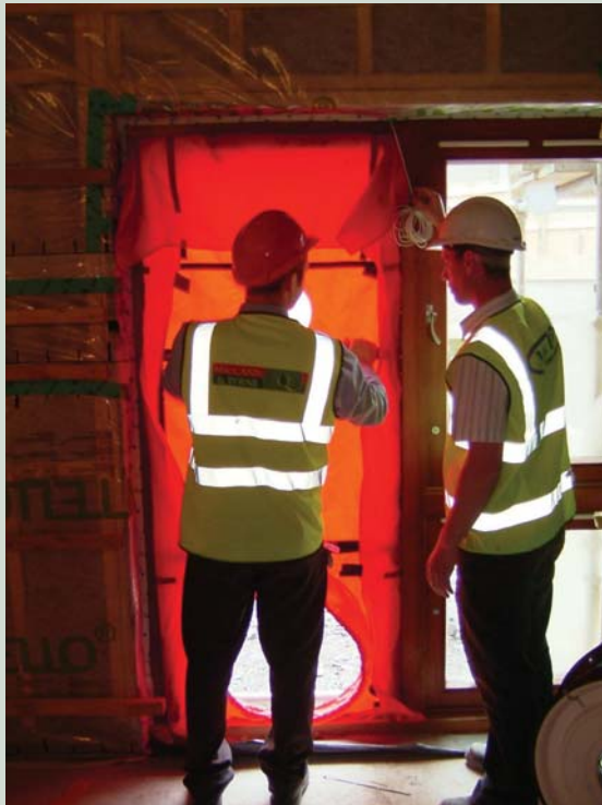
A blower door depressurisation test (left) was carried out on the first bedroom to be completed and this confirmed the airtightness details were being achieved without any problems. When the whole building was tested at Practical Completion an excellent 1.36 ac/hr at 50 pascals pressure was achieved.
