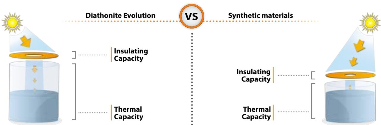
The insulating capacity (thermal conductivity) lessens the intensity of the incoming thermal wave.
