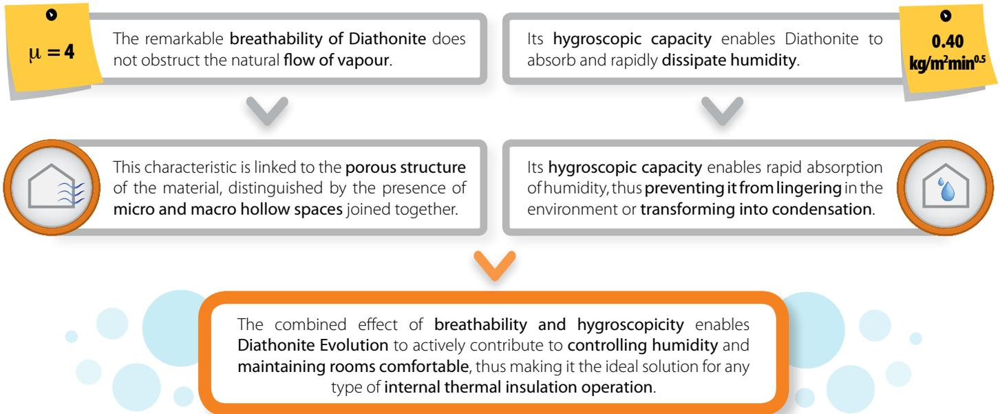
*Detail of the hygroscopic capacity of Diathonite, which can absorb and dissipate the humidity it comes into contact with, preventing it from lingering in the environment and giving rise to condensation and mould.*
