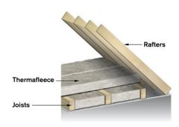
Where a low vapour resistance membrane is used, take insulation over the wall plate to meet the wall insulation and push tight against the breather membrane. Refer to the membrane manufacturer for guidance on eaves ventilation.
