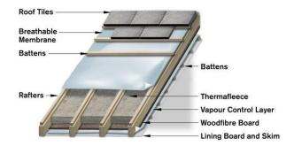
Obstructions to the roof plane should have ventilated air spaces top and bottom of each rafter to maintain the air flow in the rafter.
