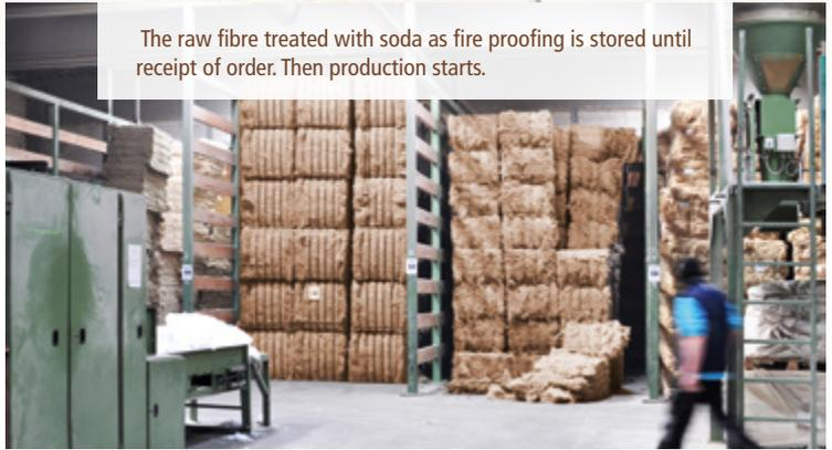
The raw fibre treated with soda as fire proofing is stored until receipt of order. Then production starts.
