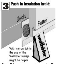
Cut off in corners and re-apply. For close connection upset joints in the corners.
