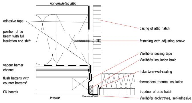
\*If battens are not flush, the adhesive strip must be securely glued to the shift. The Wellhöfer sealing tape should not be glued onto the battens but tightly and securely onto the first adhesive tape.
