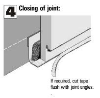
Glue sealing tape to lining bar all over.
