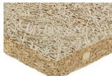
CELENIT RA is a thermal and acoustic insulation board, specific for roofing insulation, consisting of mineralized spruce wood wool bound with grey Portland cement, reinforced with three wooden strips. Wood wool is 2 mm wide.
