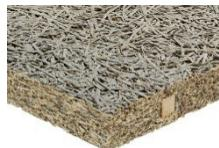
CELENIT R is a thermal and acoustic insulation board, specific for roofing insulation, consisting of mineralized spruce wood wool bound with grey Portland cement, reinforced with three wooden strips. Wood wool is 3 mm wide.
