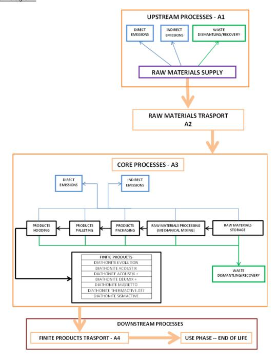
At the end of the mixing time, each product is put inside the related bag, stacked inside the pallet and protected by mean of polyethylene film.
