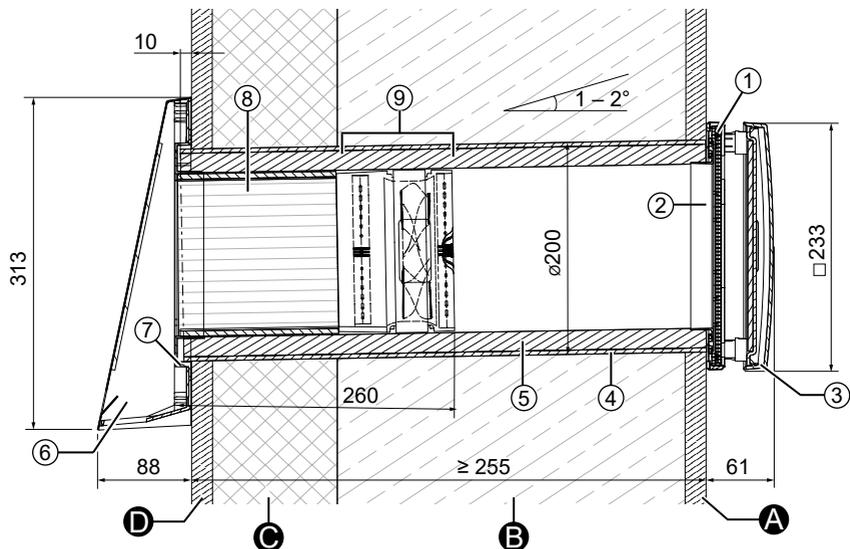
Figure 3: Sectional drawing of the iV14-Zero ventilation device
