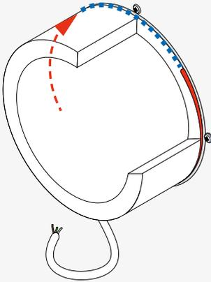
► Shorten the sound insulation lining on the inner wall side with a cutter so it is flush with the wall sleeve.
