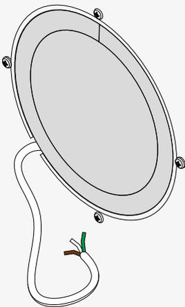
⇨ The sound insulation lining is inserted.
