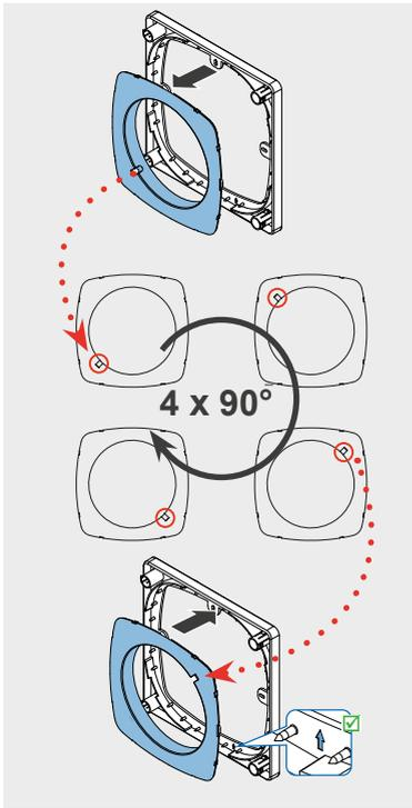
▶ Remove the Flair Zero insert by unhooking it on all 4 sides.
