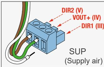
In paired operation, one reversible fan starts in extract air mode, the other in supply air mode. This start direction is determined by the different connection sequence of the three fan BUS cables in the plug-in connector.
