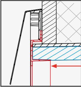
► Make sure that the sound insulation lining made of Inventin is pushed into the ring insert on the weather protection hood.
