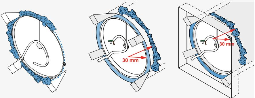
**!** Take care **not** to damage the connecting cable on the interior wall.
