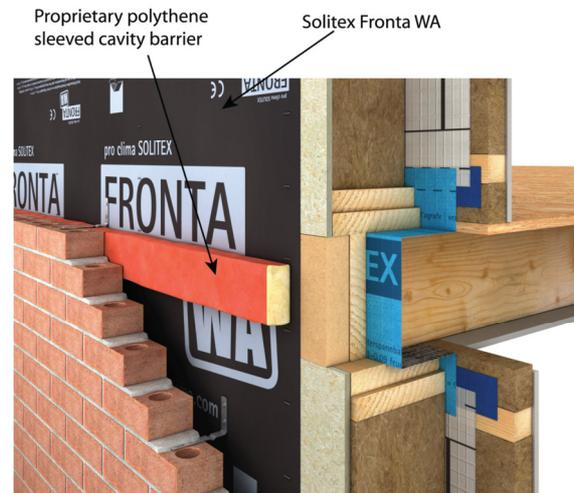
Figure 4: At Cavity Barriers
