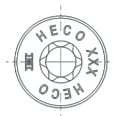
Head markings for d = 7.0 bis 12.0 mm all head types Head types without lettering possible.
