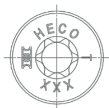
Head markings for d = 6.0 to 12.0 of types: flat countersunk head. Specified type without lettering possible too.
