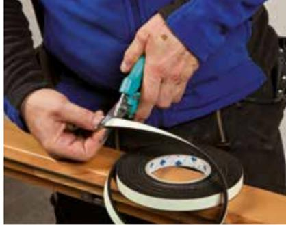
Roll off a length of CONTEGA FIDEN EXO and cut off the overcompressed start of the tape (approx. 2 cm; 3/4").
