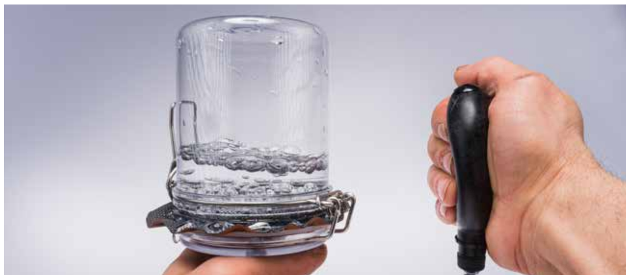
This simple test illustrates the problem with the older technology: the membrane has micropores that air can flow through. If the surface tension of the water droplets is reduced, the membrane can allow water to enter from the outside.
